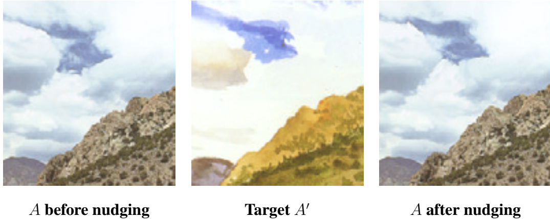
Figure C.3: In order to get images into close correspondence, we interactively deform the input A image in order to match the shape of A' . Note that, after editing, the mountain silhouette in A matches A' much more closely.
