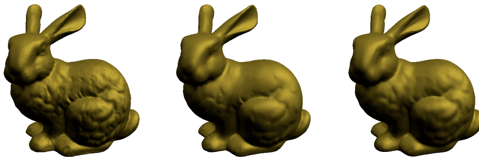
Figure 6: Denoising the reparameterized Stanford bunny mesh. (71 thousand triangles, 145 thousand after parameterization). From left to right: the reparameterized mesh; denoised by our algorithm; by anisotropic geometric diffusion method.
